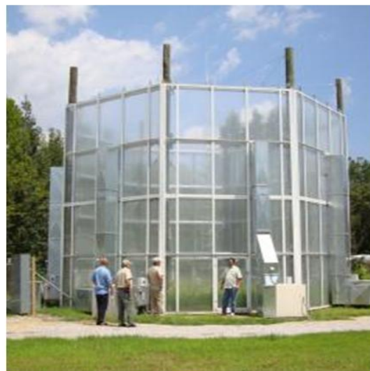
Full-scale prototype of the enclosure for testing evaluation and continued improvement constructed at ORNL.
